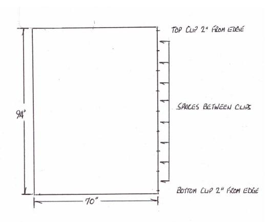
S/S Installation, Filled CMU, 40 PSF, 6 Ft span, Anchors/Clips 12" on center. 94" height requires 9 Anchors/Clips.
